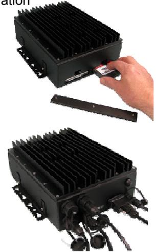
Danny Samaroo, Small PC's Technical Support Manager said *"We used both our temperature chamber and vibration table as part of the testing for the SC240ML, but I had the most fun using a fish tank for our phase one waterproof testing. It was impressive to see the SC240ML unit running while submerged in salt water. The chassis is assembled with gaskets, top and bottom, using 32 stainless steel screws to insure a tight and complete waterproof seal. "*
